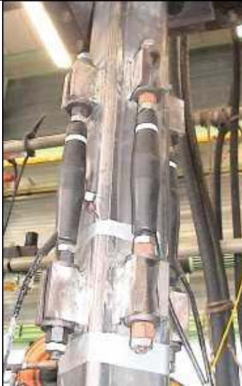
Figure 6: strain sensors mounted on a tube
