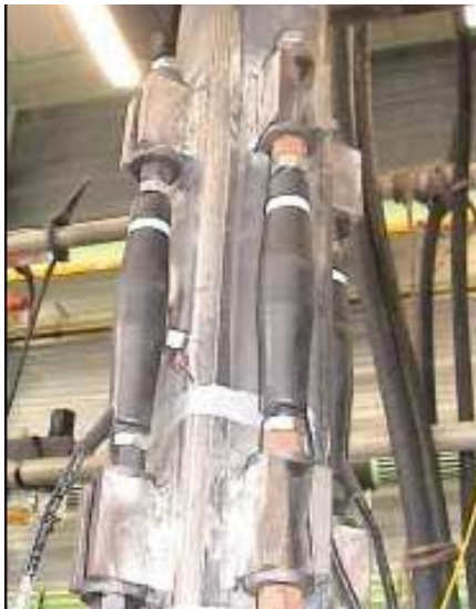
Figure 4.3 - Strain sensors mounted on a testing tube
