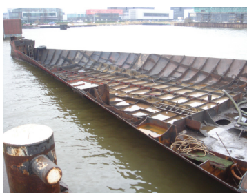
In-water ship dismantling reduces expensive dry-dock time
